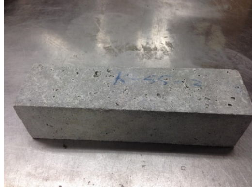
(b) 3"×3"×11.25" specimen (concrete)
