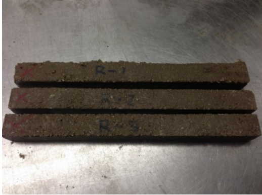
(a) 1"×1"×11.25" specimen (epoxy grout)
