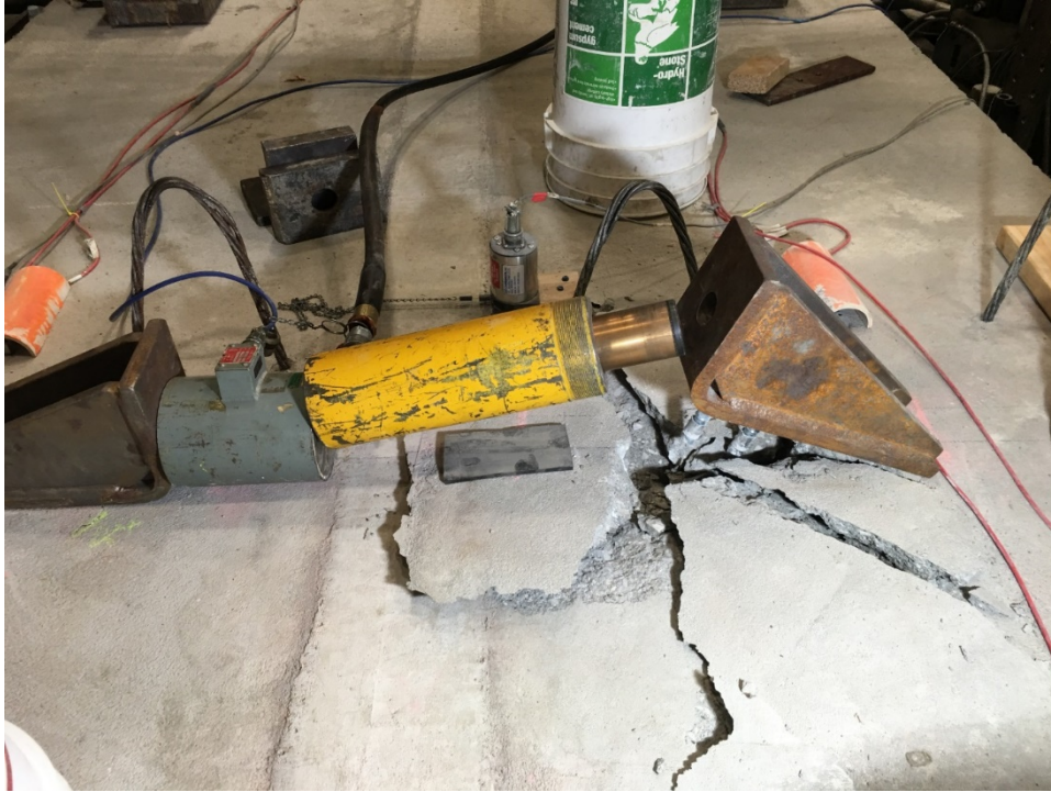
Figure 5-12 Crashed Box Girder due to Horizontal Load
